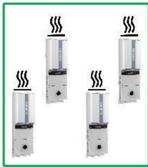
Figure 0-2a Recommended Arrangement For installation of AURORA Inverter
