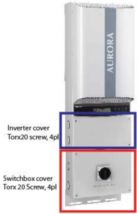
Figure 6:01- Location of Front Access Panels
