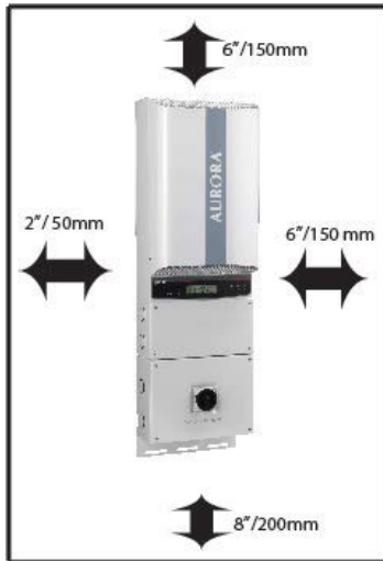
Figure 0-1 - Minimum Clearances around the AURORA Inverter
