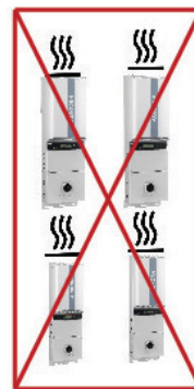
Figure 0-2b Unacceptable Arrangement For installation of AURORA Inverter
