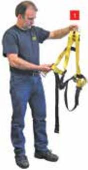
1. Hold at dorsal D-ring, and Fully inspect harness according to specifications of this instruction manual. Ensure all straps are not twisted and all buckles are unfastened.
