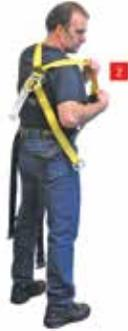
2. Place harness shoulder straps over shoulders. Ensure dorsal D-ring faces out, and is adjusted to rest between the middle of the shoulder blades.
